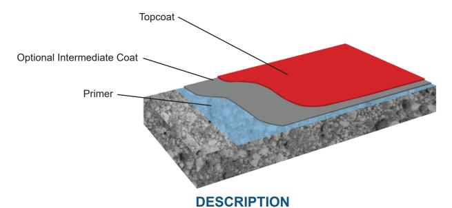
**KEY RESIN COMPANY** formulates a variety of epoxy and polyurethane coatings specially designed to protect floors from various degrees of chemical attack and abrasion. **KEY THIN-FILM SYSTEMS**, typically installed at 6-15 mils thickness, provide a brighter environment with improved cleanability over concrete surfaces. Review the requirements of your facility with the product data to select the finish that best meets the needs of the application.
