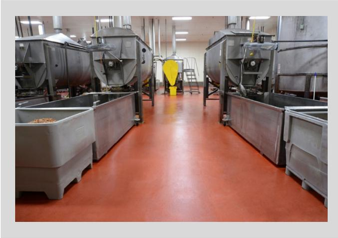
In addition, bacteria build up on the factory floor will be minimized as Flowfresh includes the unique silver-ion additive Polygiene® which inhibits the generation of up to 99% of bacteria on the floor's surface.
