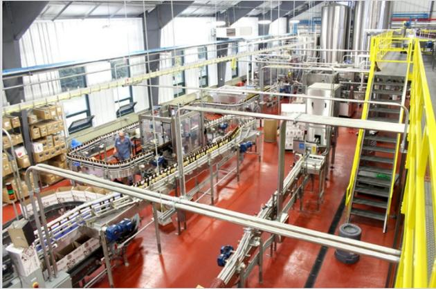
As the building was a new construction shot blasting was required in order to prepare the concrete substrate for the application process. 13,500 sq.ft. of Flowfresh SLB mortar system was then installed in the new cold storage, production, packaging and receiving area, with a full aggregate broadcast so as to provide a high level of slip resistance.
