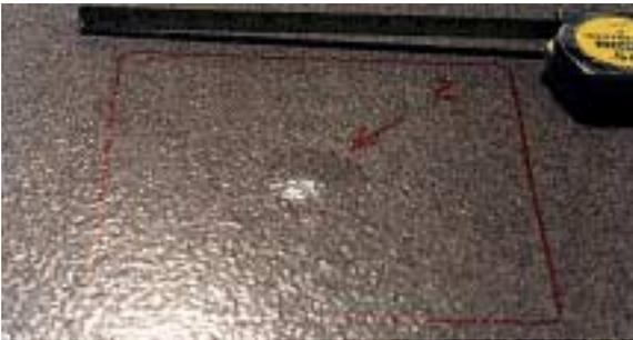
*Moisture vapor transmission failure of epoxy quartz system.*
